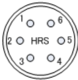
Terminal alignment (Connector bonded surface view)
